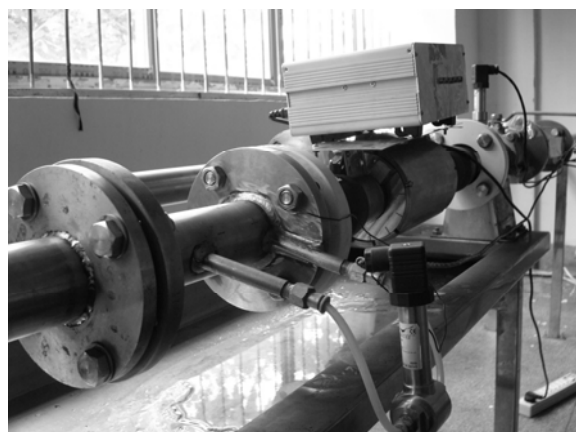
(a) Venturi tube and differential pressure sensor
